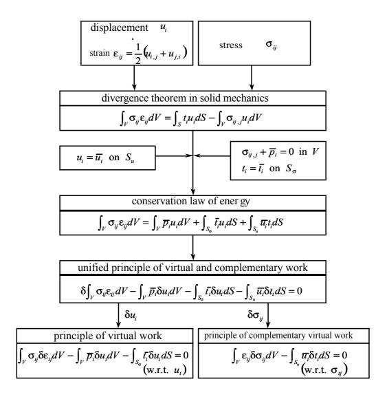
Fig.2 Process for proposing the unified principle of virtual work and complementary virtual work
